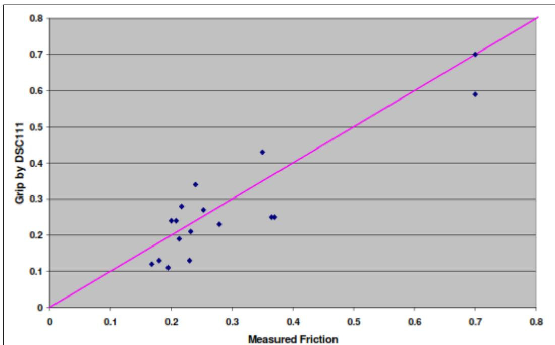
Figure 1 – Correlation between DSC111 Grip value and measured friction
