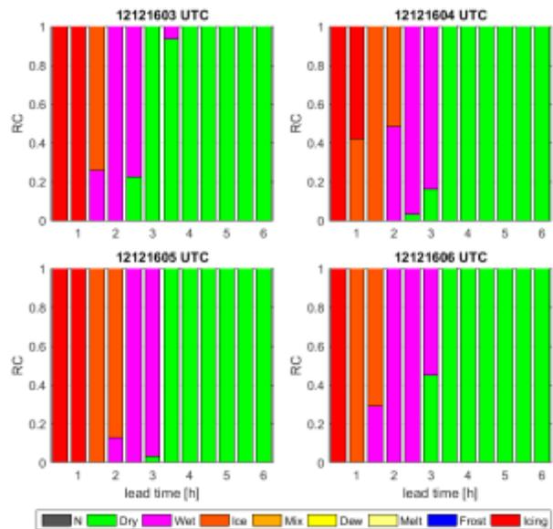
**Figure 6.** Statistically processed ensemble forecasts of road weather conditions. The vertical axis shows the probabilities, the colours indicate the RSC and the horizontal axis is the lead time. The METRo-CZ model recognizes 8 RSC (dry, wet, ice/snow, mixture of water and ice/snow, dew, melting ice/snow, frost and icing rain) and “not known” (N).
