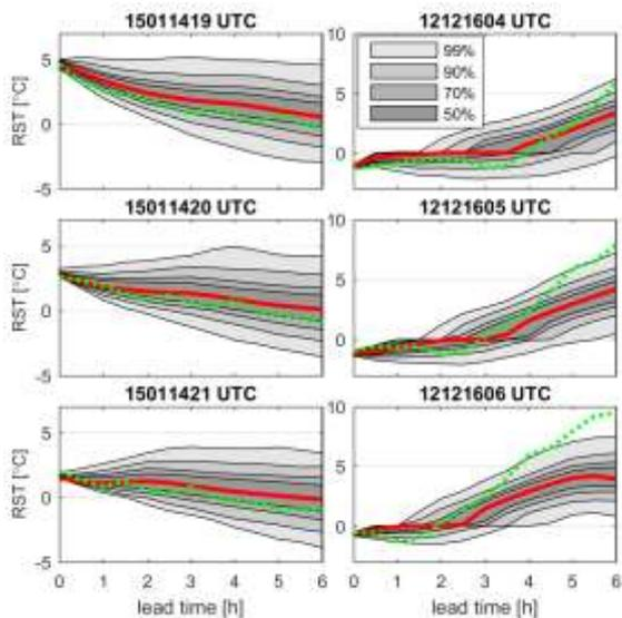
**Figure 5.** The ensemble forecasts of the RST for RWSs K013 (left column) and P004 (right column) for the lead times in hours. The full red and dashed green curves show the deterministic forecasts and observed data, respectively. The grey areas denote the intervals for probabilities 99, 90, 70 and 50% that the RST will be within that interval.
