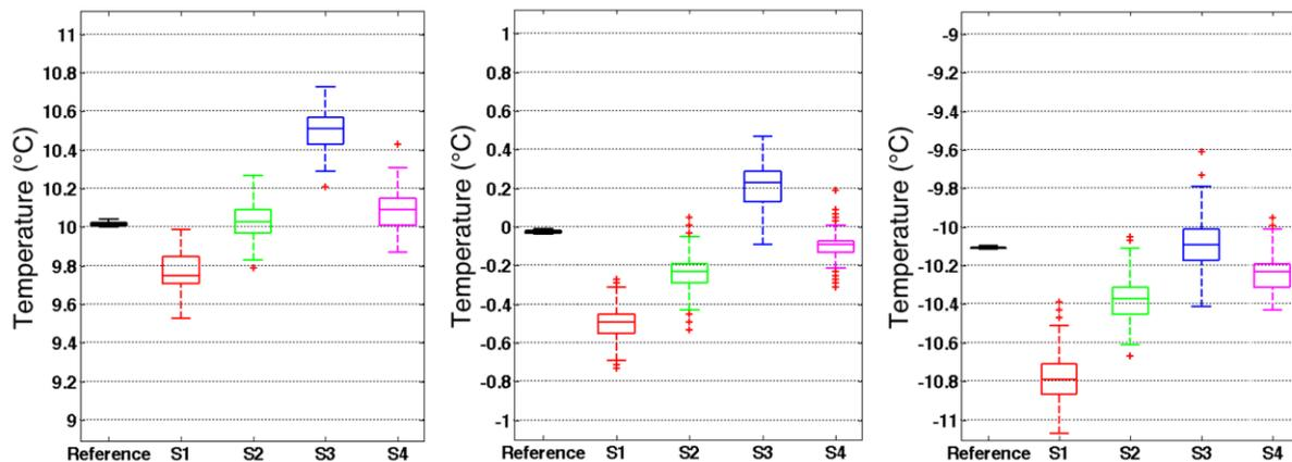
Figure 4: Box plot summary of temperature readings at three different chamber temperatures ( $+10\text{ }^{\circ}\text{C}$ ,  $0\text{ }^{\circ}\text{C}$  and  $-10\text{ }^{\circ}\text{C}$ ) by the reference thermistor and four prototype sensors. Each box represents data collected over 1 hour.
