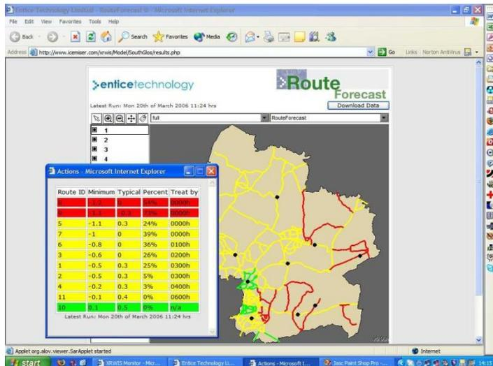
Figure 1: Screenshot of XRWIS. The fundamental difference between RWIS and XRWIS was the change from a reliance on thermal mapping to an increasingly high resolution modelling approach. Instead of running a model for a handful of outstations, the model was now run for thousands of sites across a network just metres apart. This is how these maps are produced – these consist of point data and not the line data which is how the visualisation appears.
