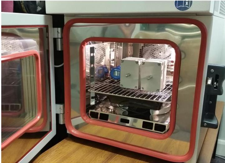
Figure 3: The Weiss WKL 34 climate chamber. Inside are the four test sensors mounted above the slab of asphalt into which the reference thermistor is embedded.
