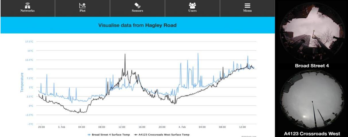
Figure 6: A screenshot of the web application being used to compare time series data from two of the sensors deployed along Hagley Road Birmingham. The sensors are ~3.5 km apart. The adjacent fisheye lens photographs illustrate the differences in sky view factor at the two locations.
