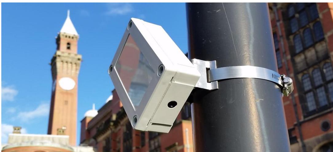
Figure 2: Prototype road surface temperature mounted, as operationally, on street furniture adjacent to a road. The small black hole is the MLX90614 aperture, which is aimed at the road surface.
