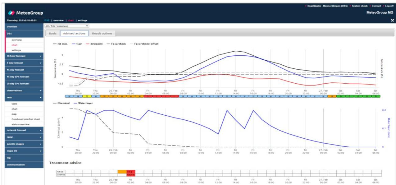
Detailed road weather forecast for a route and the resulting treatment advice from DSS at the bottom
