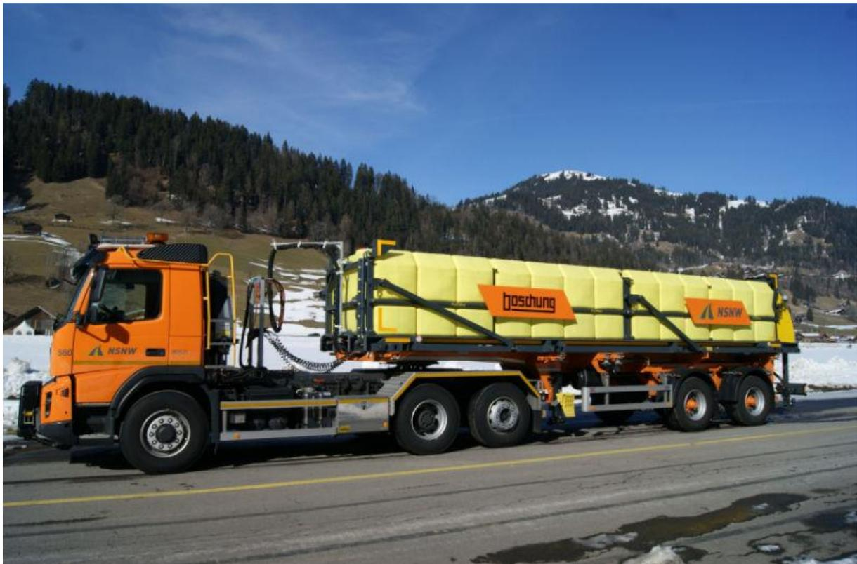
**Picture 2:** Winter service manager has to decide, when and with how many vehicles to start the necessary treatments (here a spreader with 22.000 l brine)
