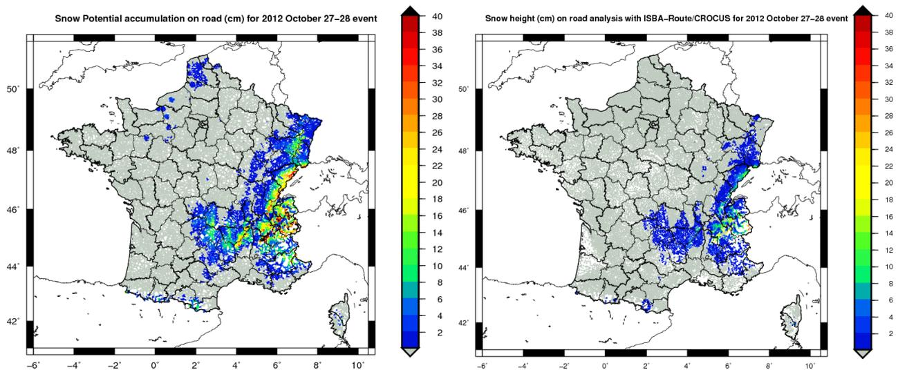
Figure 2. Comparison for the October 27-28, 2012 event of the snow potential on the road (left panel, road network scale) and the analysis of snow height on road done with the ISBA-Route/CROCUS model (right panel, French cities scale).
