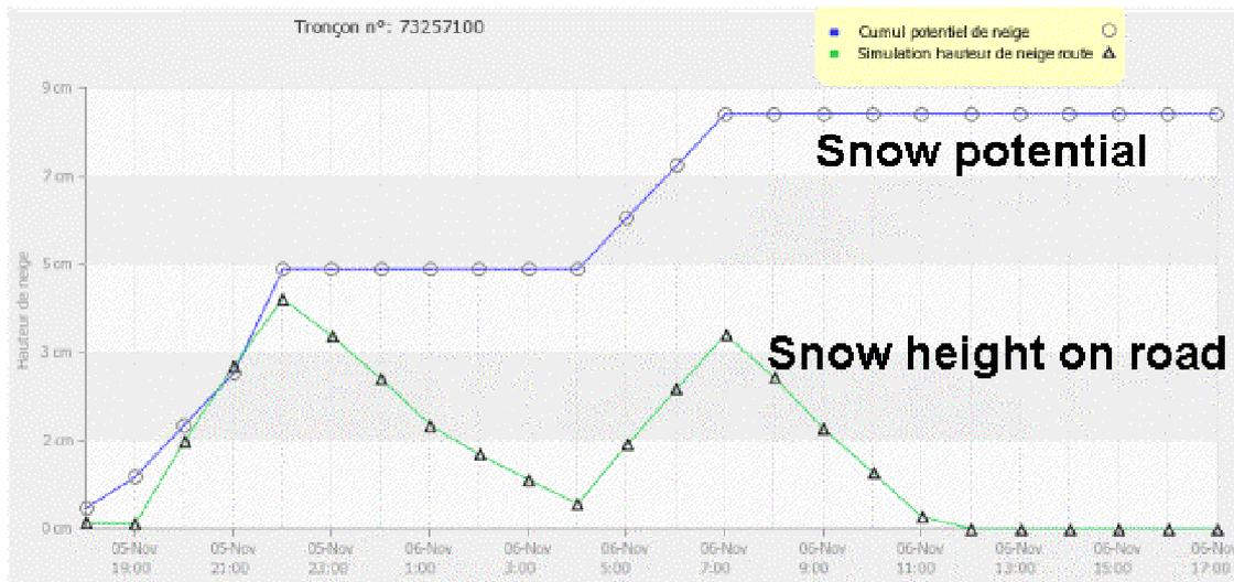
Figure 4. Example of time evolution differences between the forecast of snow potential on the road (blue line) and the forecast of snow height on road done with the ISBA-Route/CROCUS model (green line) for a French road section, for the November 6, 2013, 16h UTC forecast.
