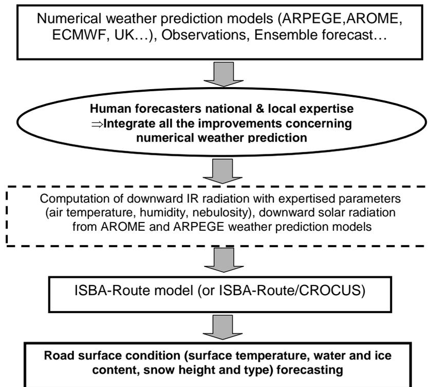
Figure 1. Simplified diagram of the PEIR Météo-France operational system for road surface conditions forecasting.
