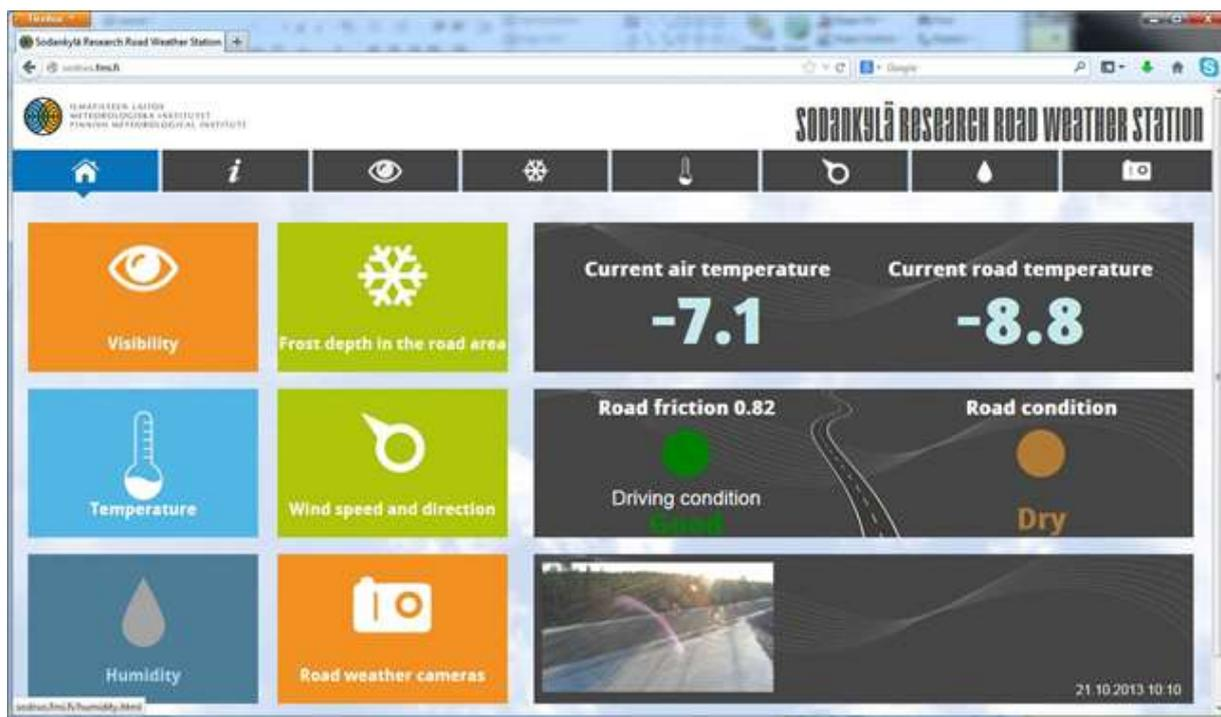
Figure 2. Road Weather Station user interface in the Internet (and in a smart phone).
