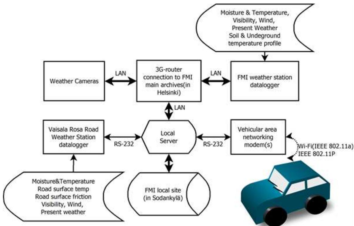
Figure 1. Communication entity of RWS/RSU.
