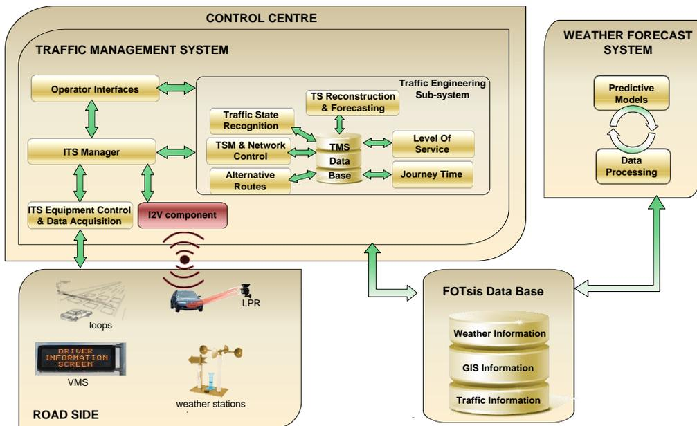
Figure 1. FOTsis highway control center structure.
