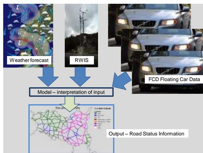
Figure 1. RSI – for winter road conditions, where input from different sources makes it possible to improve the information to maintenance operators.
