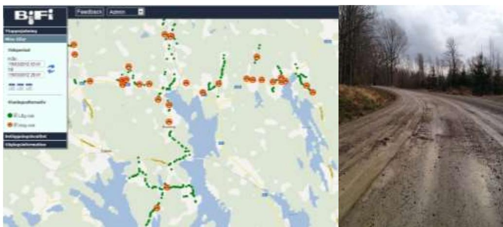
Figure 2. Display of frost thaw situation and example of how a typical gravel road can look like during these conditions..
