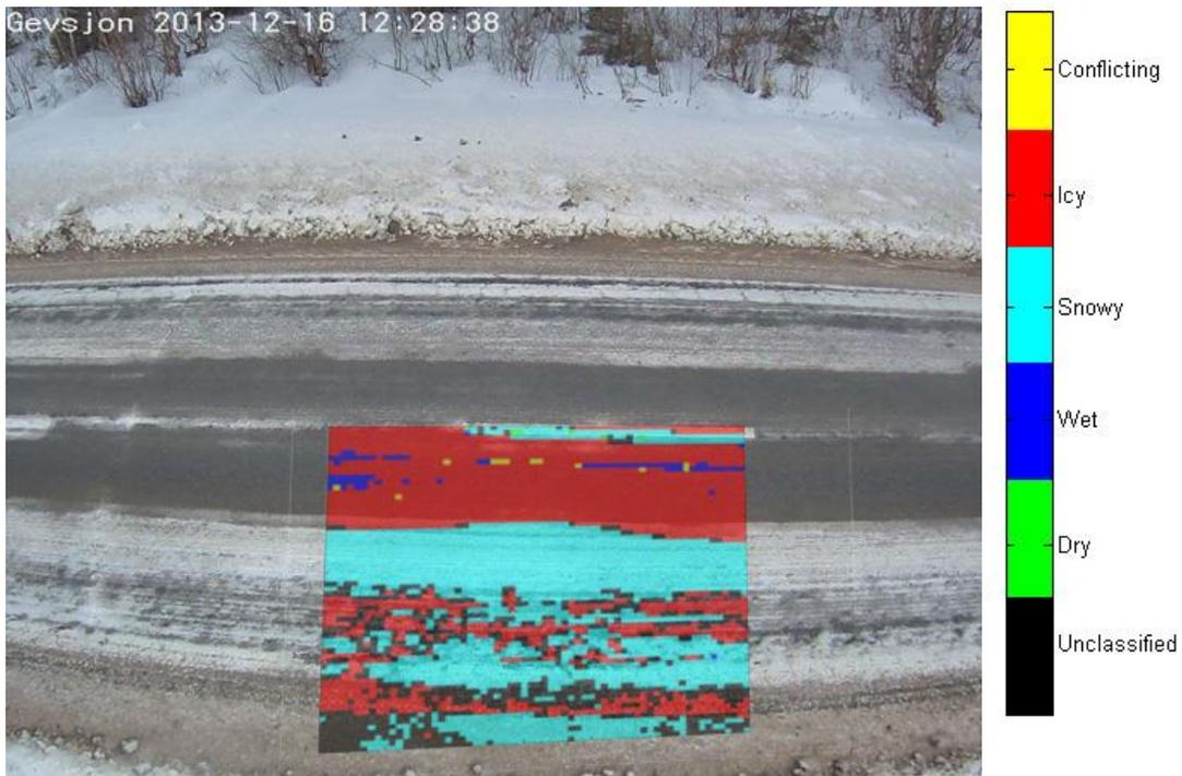
Figure 6. Background image taken with ordinary visual camera system. A classification image made from NIR camera data is overlaid on a part of the visual image. It can be seen that different road conditions are detected on the road surface.
