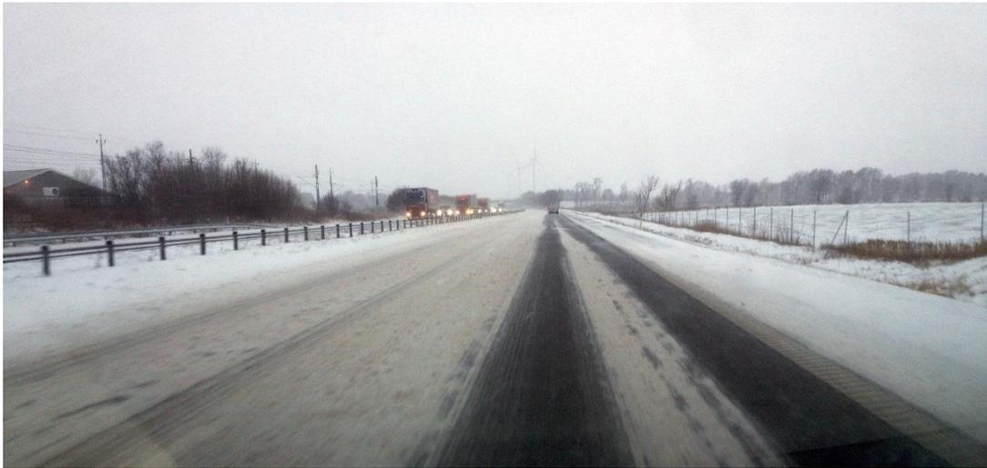
Figure 1. Picture of a road lane section where there are very different road condition in the wheel tracks and in-between the wheel tracks. There is ice in the wheel tracks and packed snow in-between the wheel tracks.
