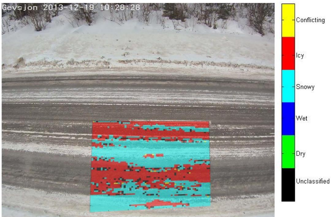
Figure 7. A classification image made from NIR camera data is overlaid on a part of a visual image. It can be seen that different road conditions are detected on the road surface.
