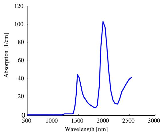
Figure 2. Water absorption in the region 500 to 2500 nm [5]. It can be seen that there are some peaks in the absorption that may be used to detect water.
