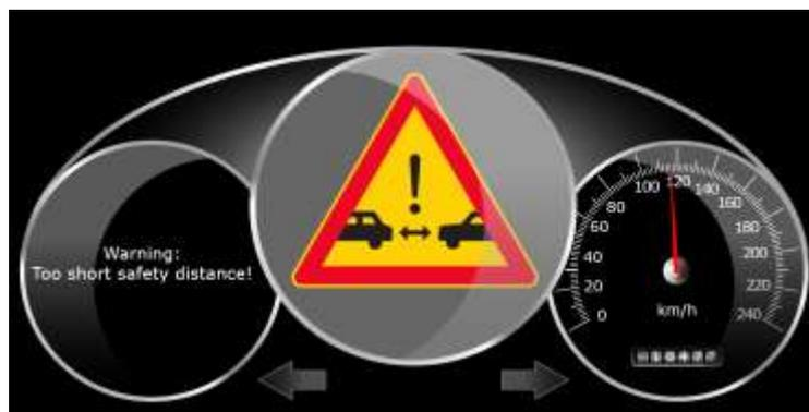
Figure 6. Screenshot of the car's dashboard in the pilot when the warning is given.
