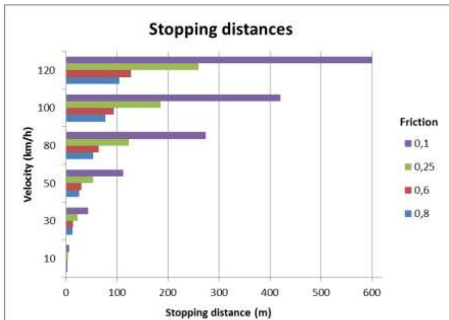
Figure 2. Stopping distances (including reaction distance and braking distance) as a function of different initial velocities and frictions.
