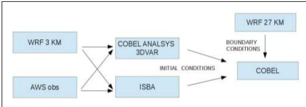
Figure 3. Flow chart of the COBEL simulations indicating the origin of the boundary and initial conditions
