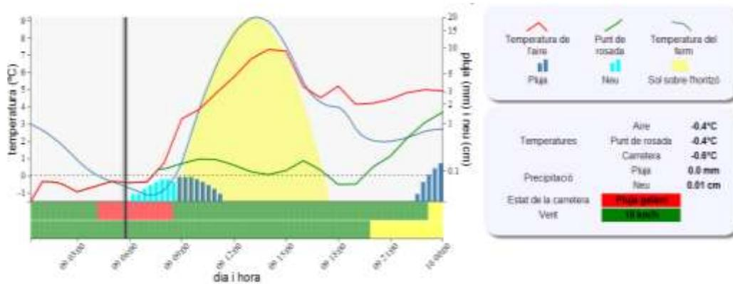
Figure 8. Example of the new graphical interface proposed that merges the information of the METRo model and CALMET
