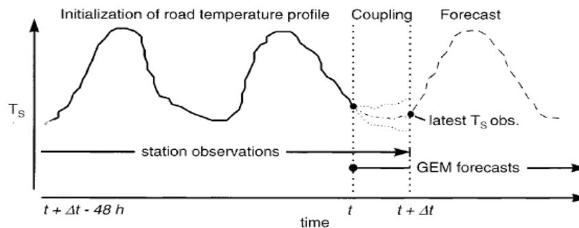
Figure 2. Structure of the METRo simulations with three phases: initialization, coupling and forecast
