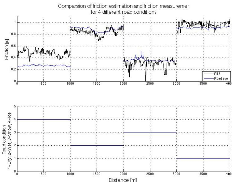
Figure 5. Comparison of friction estimation and friction measurement methods for different road conditions.
