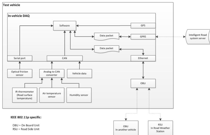
Figure 2. Description of a basic in-vehicle DAQ system setup.
