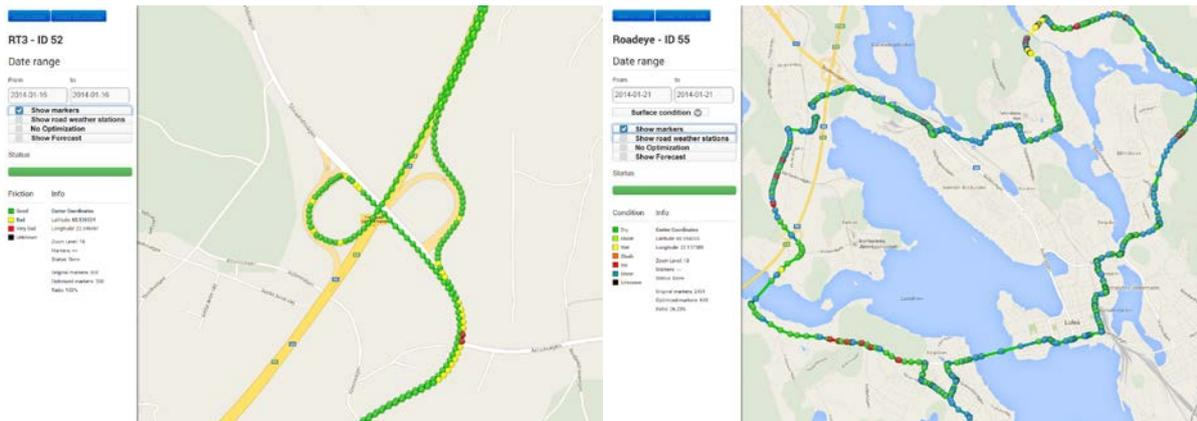
Figure 4. Friction view (RT3) on the left and surface condition view (Road Eye) on the right side.
