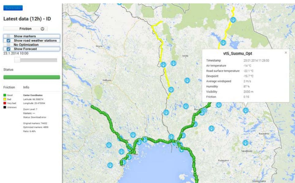
Figure 3. Intelligent Road web interface showing road weather forecast, road friction and RWS data.
