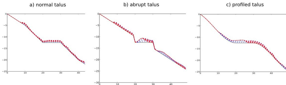
Figure 3. Snow deposition and secondary transport with three different slope profiles. Wind direction is from the reader's left.
