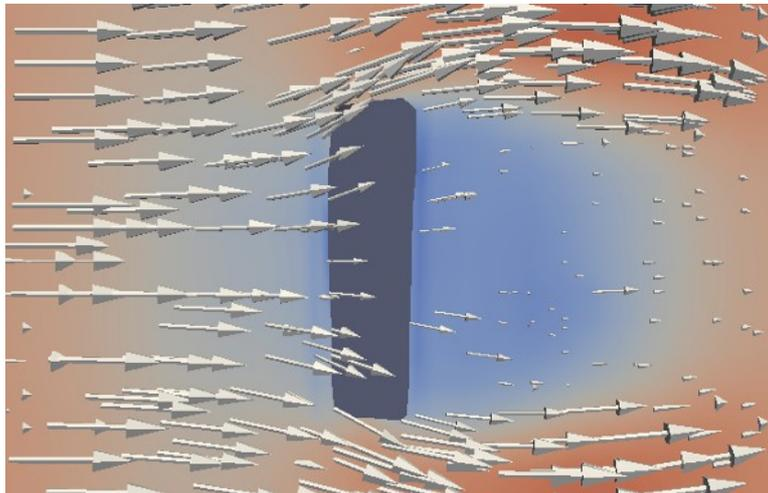
Figure 8. Airflow around a large vehicle, immobilised along the road.
