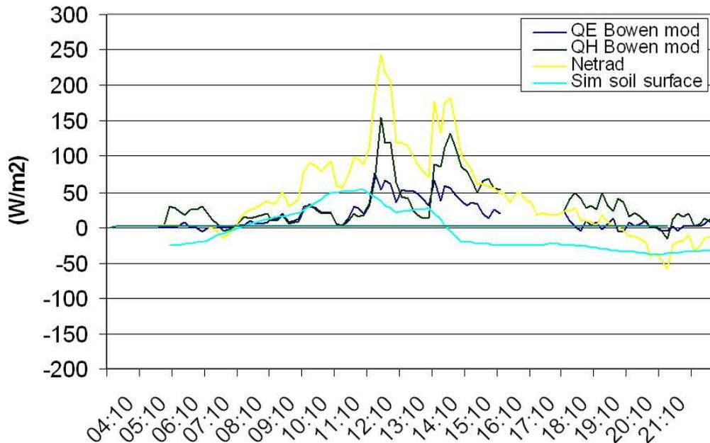
Figure 7: The energy fluxes measured using the Bowen ratio method. The data is from the 3 April, 2003.
