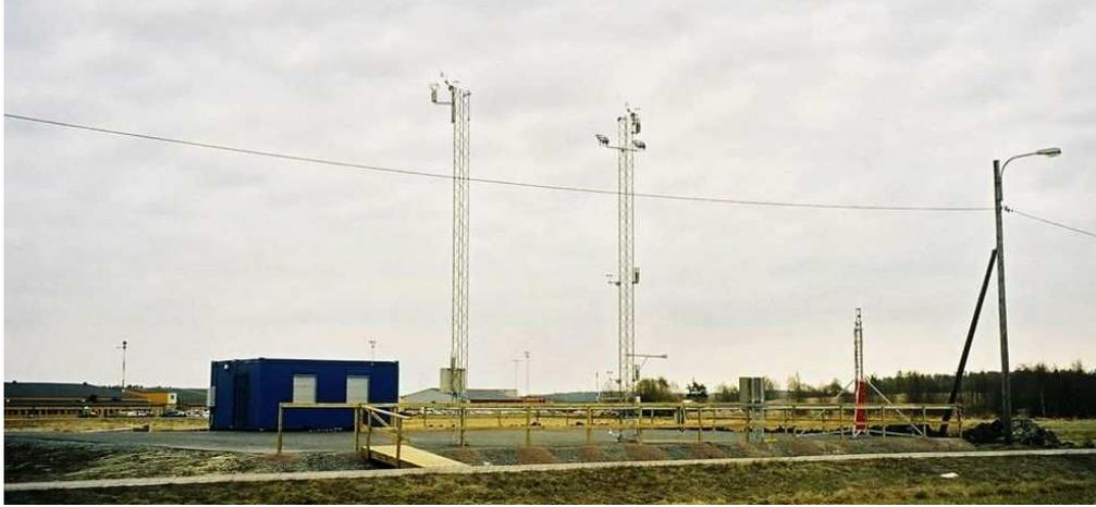
Figure 2: The asphalt surface at S ave as seen from the north-west. The RWIS-station is mounted on the left tower, while the instrument measuring the radiation components is on the right tower. The road is seen as a grey line in the foreground.
