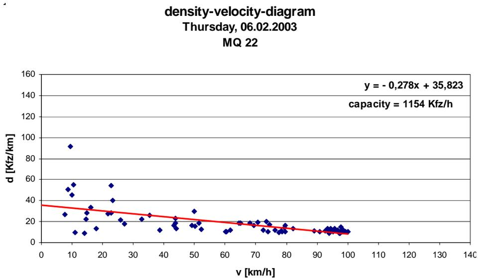
**Figure 1** Example of a d-v-diagram of a winter-related congestion –  $q_{\max}$  capacity determined
