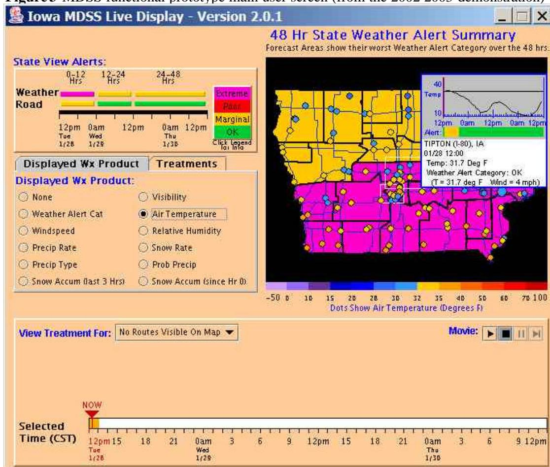
The MDSS contains a “what-if” scenario treatment selector. This means that the operator is able to modify the recommended treatment times, chemical types or application rates, and see how the road condition predictions might change.
