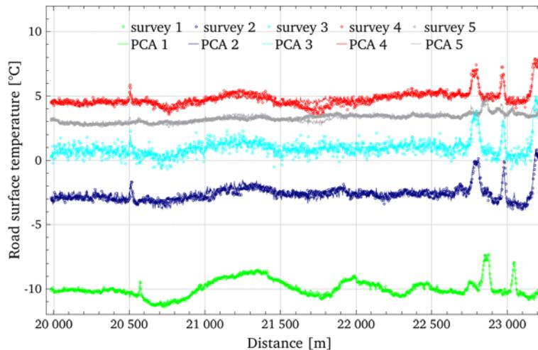
Figure 3. Comparison between raw measurements and corresponding PCA modelled fingerprints under 5°C for road section 4
