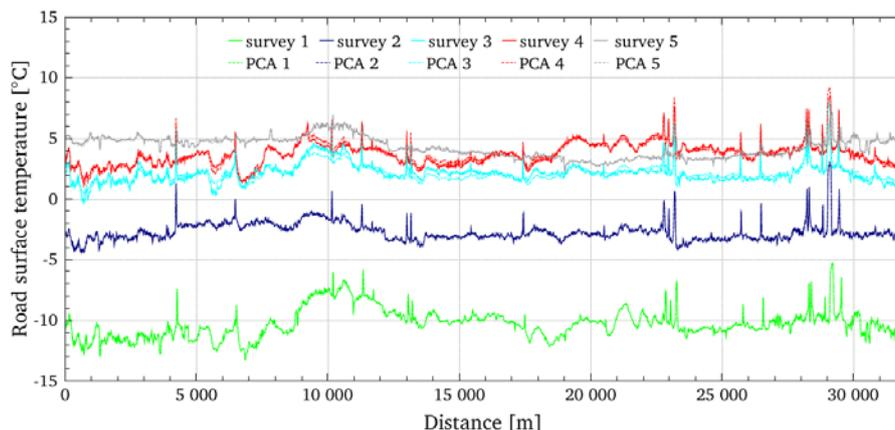
Figure 1. Comparison of raw measurements and corresponding PCA modelled fingerprints under 5°C (Case 3)
