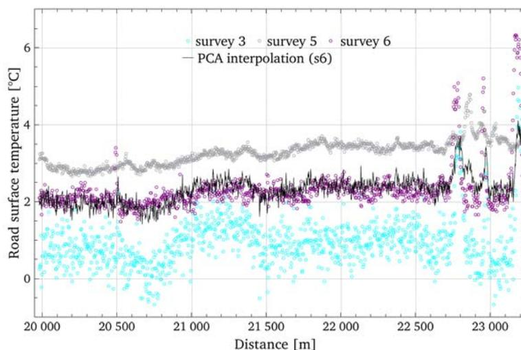
Figure 4. Comparison of survey 6 raw measurements and interpolated (“predicted”) values from PCA computations
