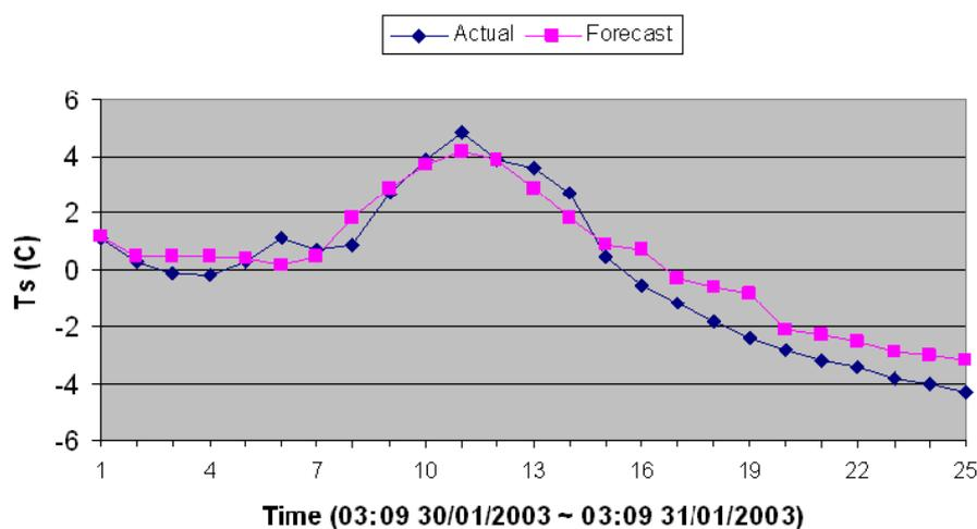
Figure 1. Comparison of nowcasts and measurements of RST at station (ID=BC004)
