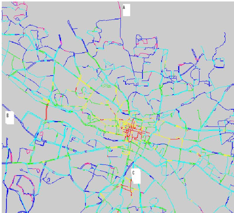
Figure 4. Measured RST distribution at Glasgow by Thermal Mapping (Extreme)
