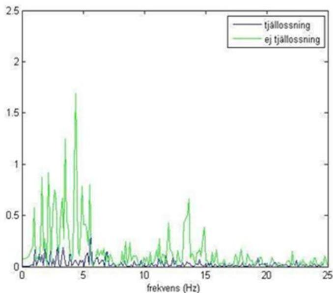
Figure 1. Detection of lateral acceleration in the vehicle reveals the road conditions.
