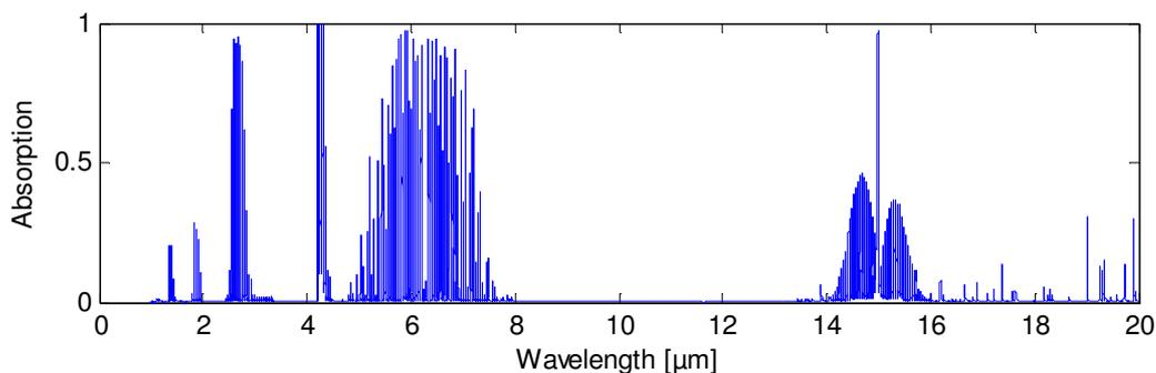
Figure 1. Absorption of IR light by common atmospheric gases. It can be seen that the atmospheric absorbance is low in some wavelength bands, for example between 8-14  $\mu\text{m}$ .
