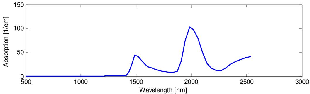
Figure 2. Absorption of water in the NIR region. Some characteristic peaks can be seen.
