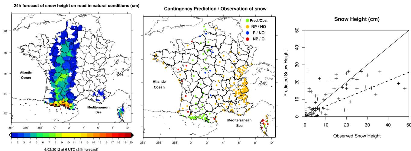
Figure 2. Results of the snow on road forecast for the 5 February 2012 event: 24h predicted snow height on the roads (in natural conditions without traffic or road treatments) (left), contingency with observations (centre) and comparison of predicted snow height on road with observed snow height on natural soils (right).
