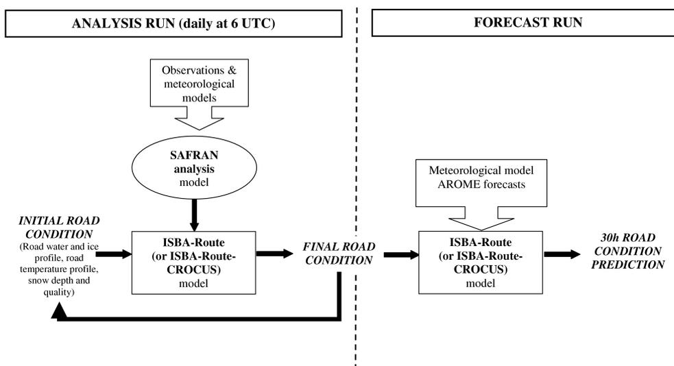
Figure 1. Simplified diagram of the AROME-ISBA-Route (AIR) road condition prediction system for the 6h UTC run with daily analysis.
