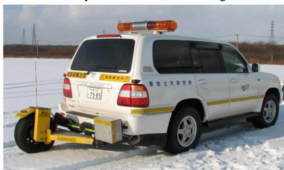
Figure 5. Continuous friction tester (CFT)
