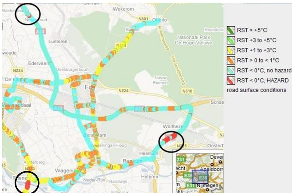
Figure 2. In this output of the MeteoGroup route based forecast for road surface temperature and condition, the critical areas (red colors within the circles) can easily be distinguished.
