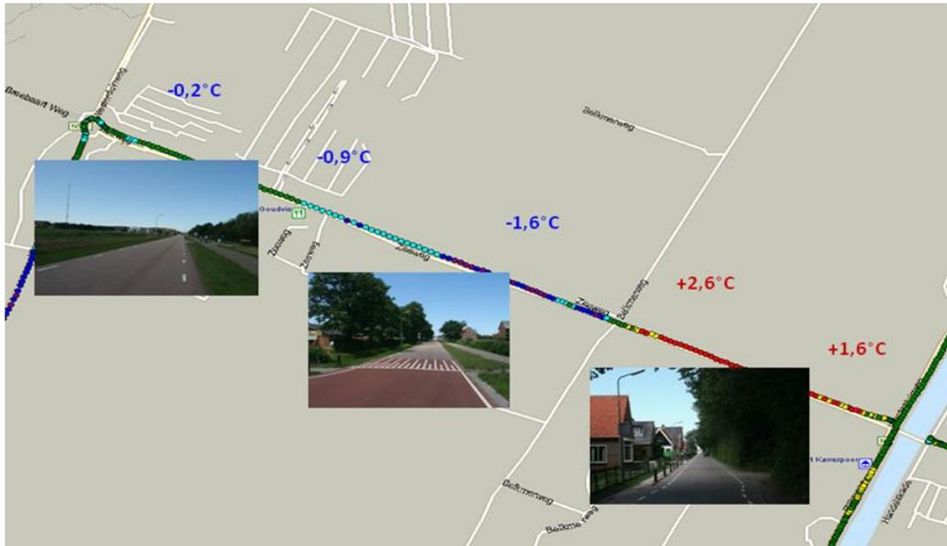
Figure 1. Infrared measurement of the road surface temperature. Sheltered areas show as higher temperatures (right side of the figure), open areas appear as lower temperatures (left side).
