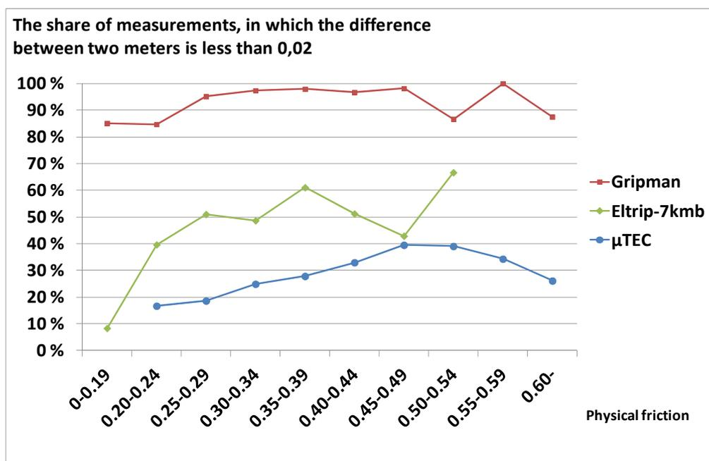
Figure 3. The share of measurements in which the difference between the results of two meters is less than 0.02.
