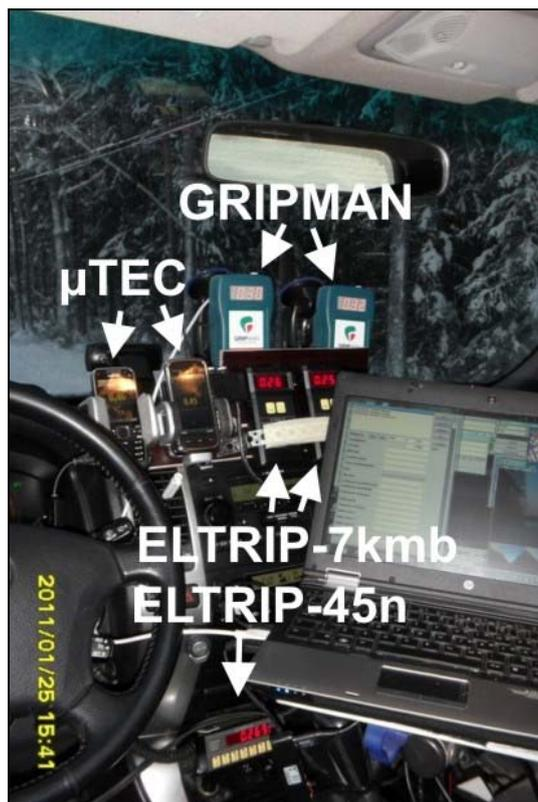
Figure 1. Acceleration sensor meters ( $\mu$ TEC, Gripman, Eltrip-7kmb) and the traditional meter (Eltrip-45n) in the vehicle
