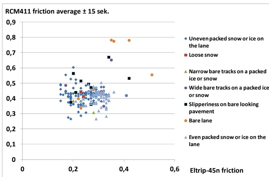
Figure 7. The RCM411 and Eltrip-45n compared on actual road conditions
