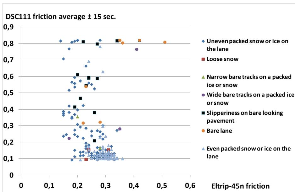
Figure 6. The DSC111 and Eltrip-45n compared on actual road conditions
