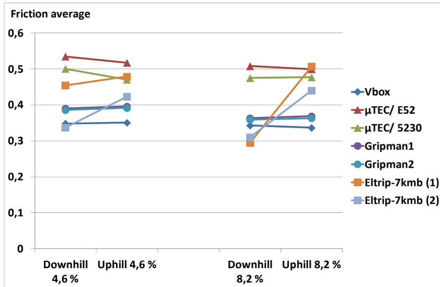
Figure 5. The ability to measure friction on a hill.
