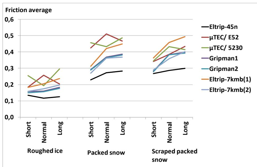
Figure 4. The effect of braking time (short, normal or long) on friction values on different test track surfaces
