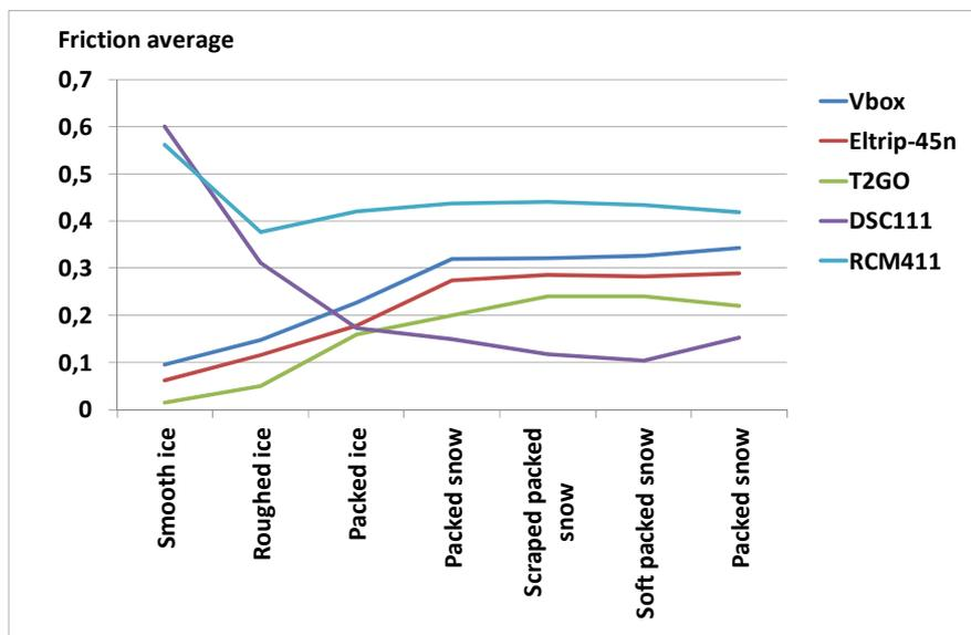
Figure 5. Optical meters and the T2GO compared with the Vbox and Eltrip-45n on test tracks
