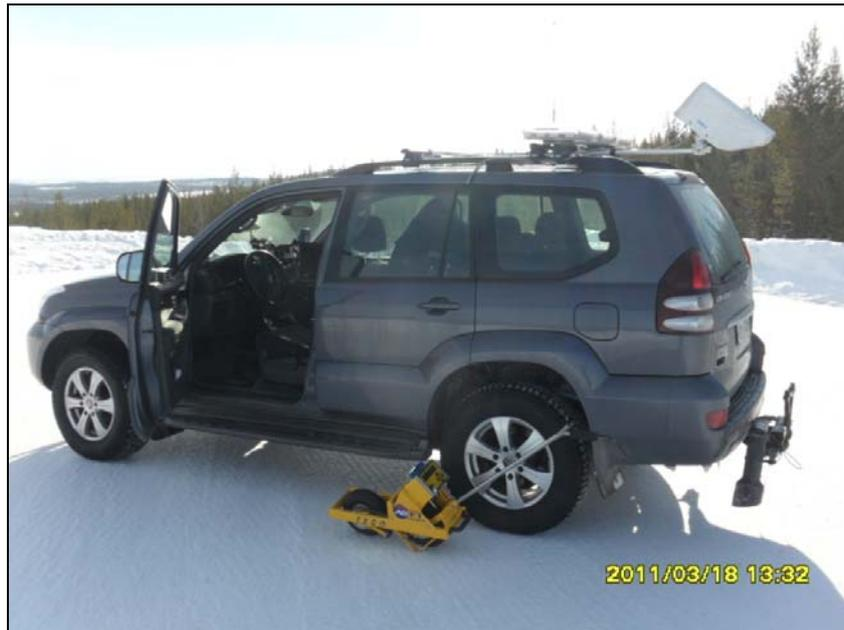
Figure 2. DSC111 (white box) on the roof, RCM411 in the towing hook, T2GO (yellow device) in front of the vehicle.
