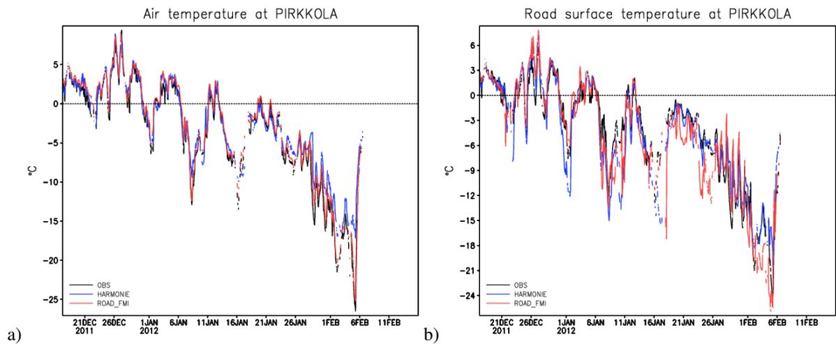
Figure 2. Observed (black line) and modelled by HARMONIE (blue line) and FMI's road weather model (red) temperatures on Pirkkola, Helsinki. Air temperature on the left (a) and road surface temperature on the right (b).
