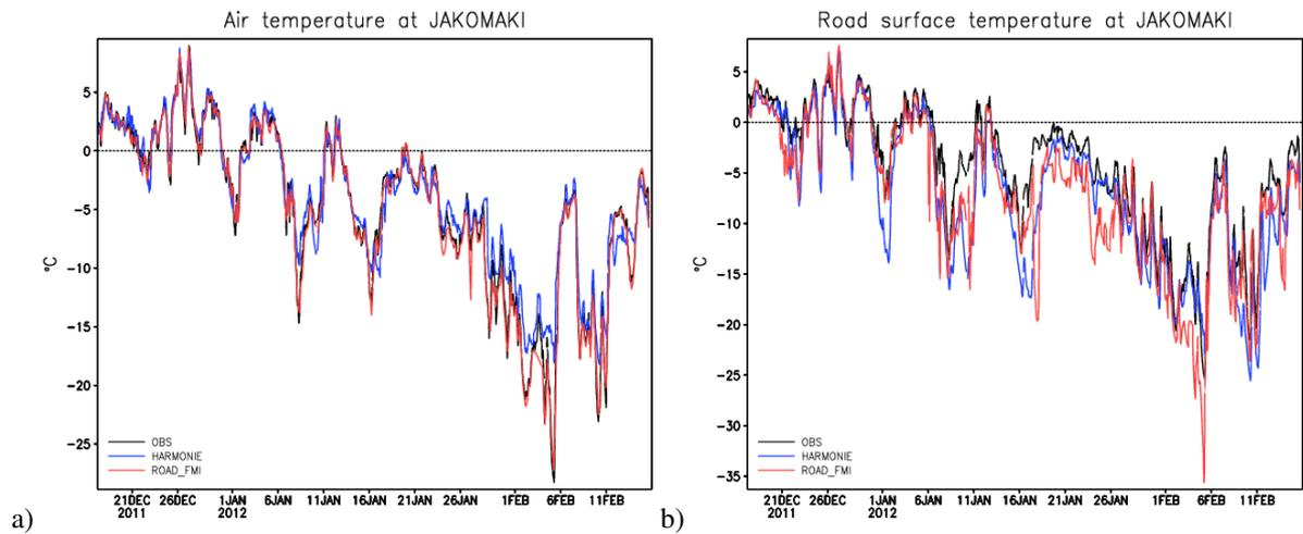
Figure 1. Observed (black line) and modelled by HARMONIE (blue) and FMI's road weather model (red) temperatures on Jakomäki, Helsinki. Air temperature on the left (a) and road surface temperature on the right (b).
