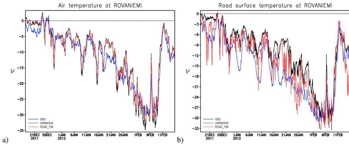
Figure 4. Observed (black line) and modelled by HARMONIE/SURFEX (blue) and FMI’s road weather model (red) temperatures on Rovaniemi. Air temperature on the left (a) and road surface temperature on the right (b).
