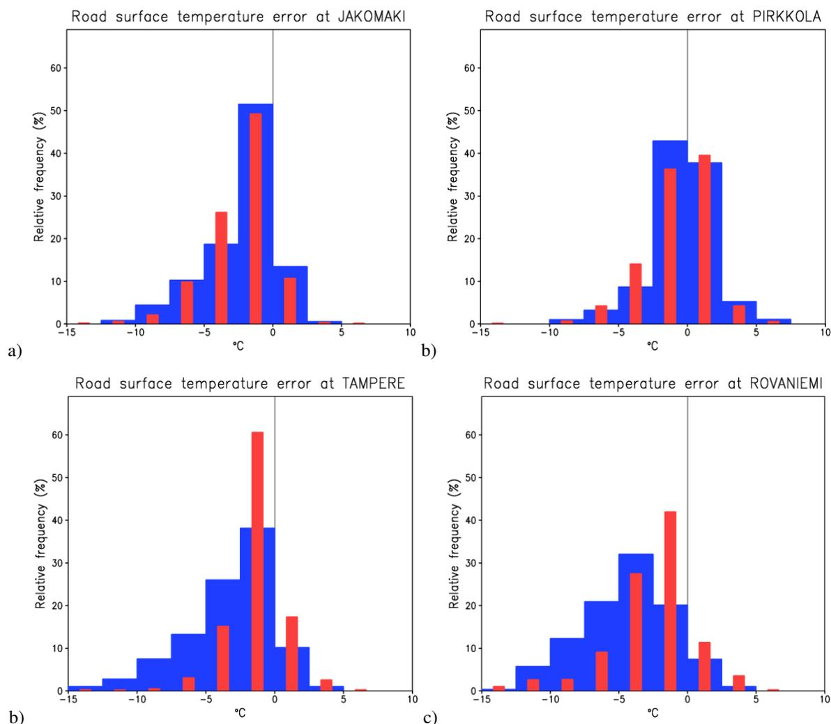
Figure 4. Road surface temperature error between modelled and observed values in four studied places; Jakomäki, Helsinki (a), Pirkkola, Helsinki (b), Tampere (c) and Rovaniemi (d), respectively. Blue columns are presenting HARMONIE/SURFEX and red columns FMI's road weather model.
