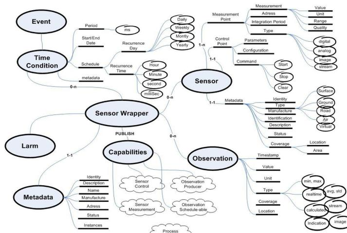
Figure 2 Sensor Data Model
