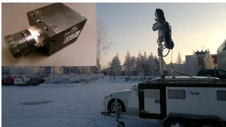
Figure 1: Road side unit (RSU) with Xenics XS-1265 NIR camera. All the test images were capture with this unit. Vehicle on background was carrying stereo camera unit.
