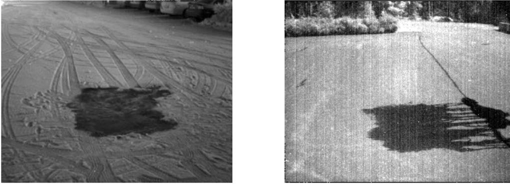
Figure 2. NIR image shows clearly the difference between ice and snow (left side). The image is taken in the winter. The moistened road surface is clearly similar than the dry asphalt road (right side). The image is taken in the summer time.
