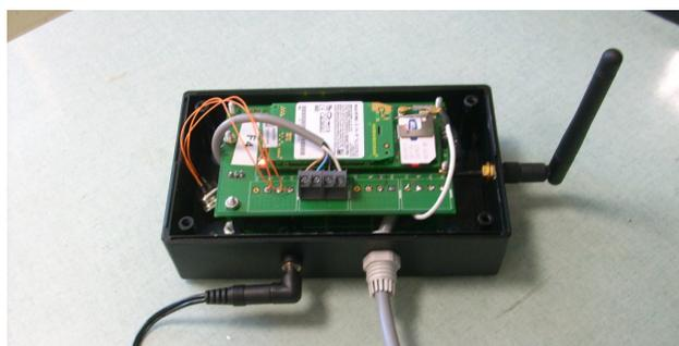
Figure 3. The GPRS based data acquisition system.
