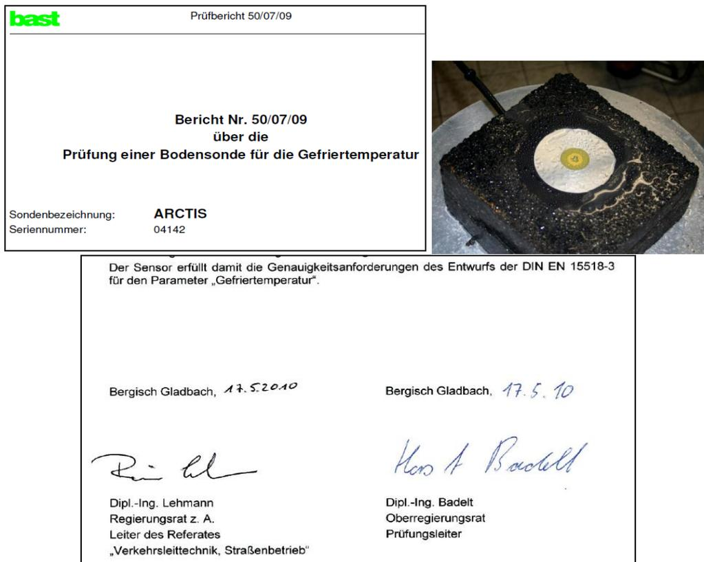
Figure 4. Excerpt of the certification report of the ARCTIS active pavement sensor from Boschung Mecatronic, stating that the sensor meets the requirements on measured freezing point temperature of EN15518-3 [2]
