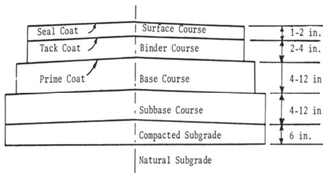
Figure 1. Typical Cross-section of Conventional Flexible Pavement
