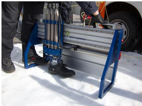
Figure 3. A slip resistance simulator developed by Finnish Institute of Occupational Health.
