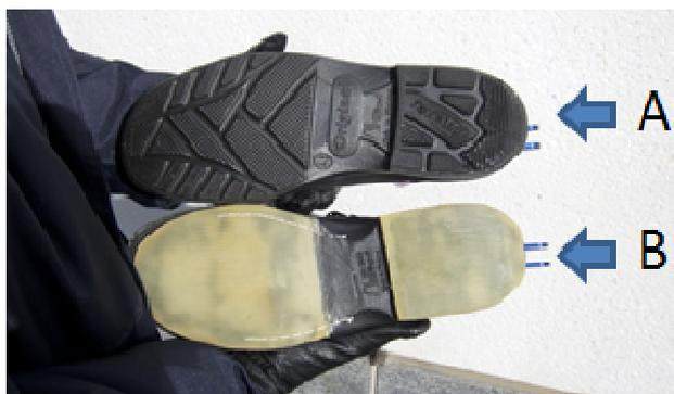
Figure 4. Shoe soles used in the slipmeter simulations; shoe A with a good grip sole and shoe B with a slippery sole.
