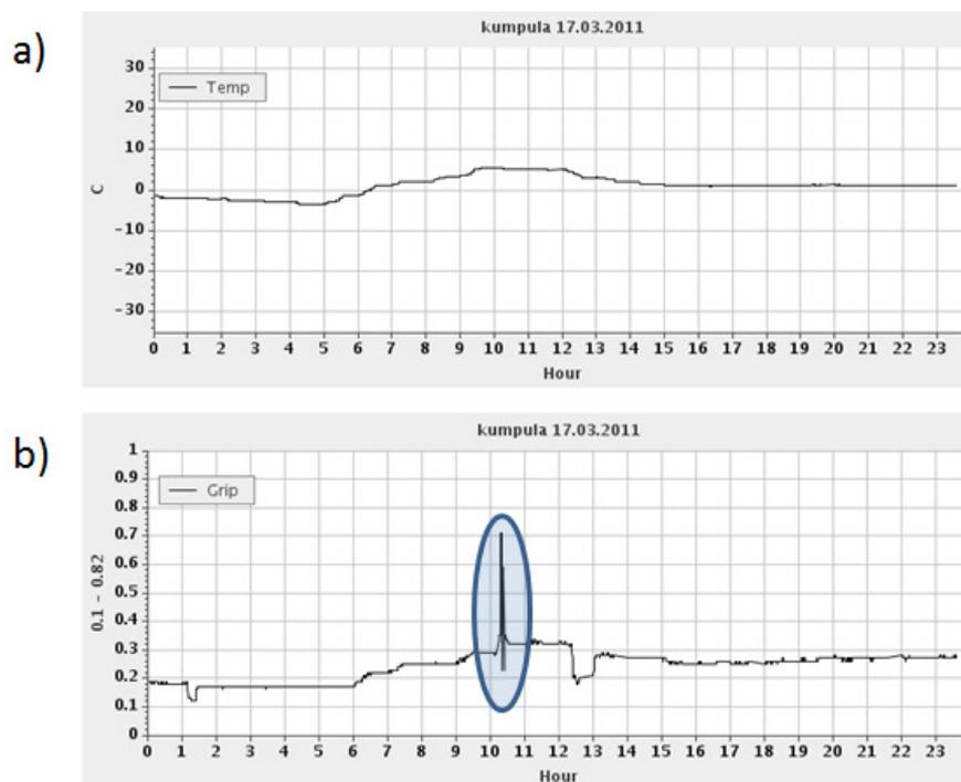
Figure 5. Observations measured by Vaisala DSC111 instrument on 17<sup>th</sup> March 2011. Upper picture measured air temperature (a) and lower picture friction (b). The blue ring is presenting the measurement time.
