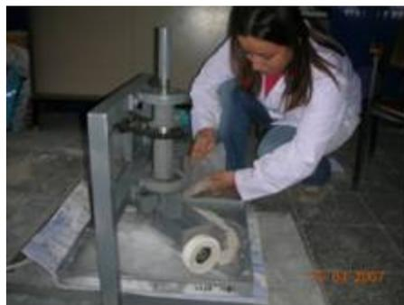
Figure 4. Placement of abrasive specimen onto ice surface
