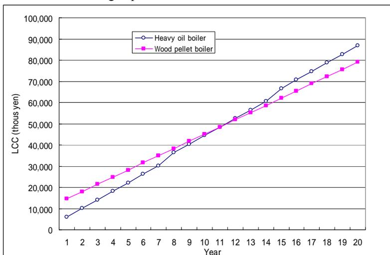
Fig.4. Comparison of life cycle costs for hot water boilers for snow melting facilities
