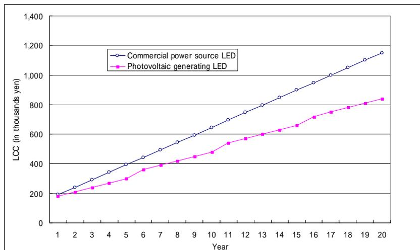
Fig. 5. Comparison of life cycle costs by different power line systems
