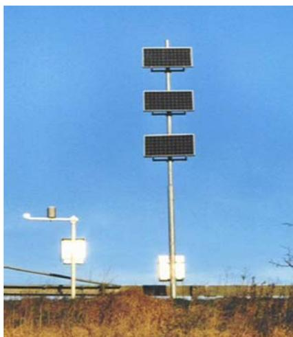
Fig. 5. Measuring station with solar cells and wireless transmission
