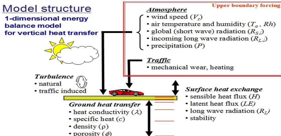
Figure 2. Schematic of the road weather model.
