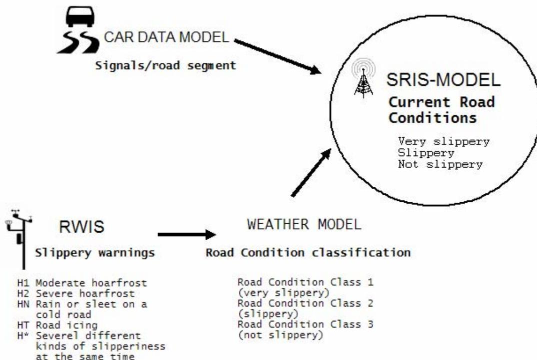
Figure 3. Sketch of how the SRIS model is built and function.
