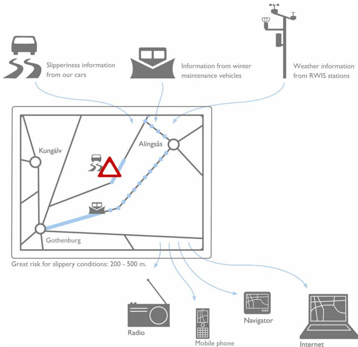
Figure 2. Schematic sketch of how SRIS is supposed to function.
