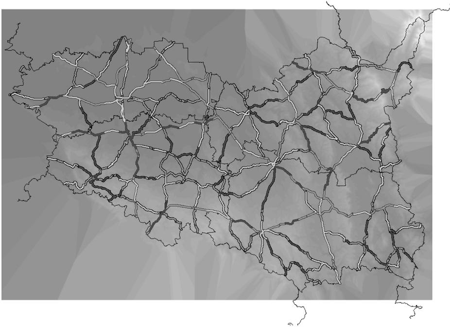
Figure 3. Map of the test area with roads divided into segments indicating different levels of slipperiness exposure.
