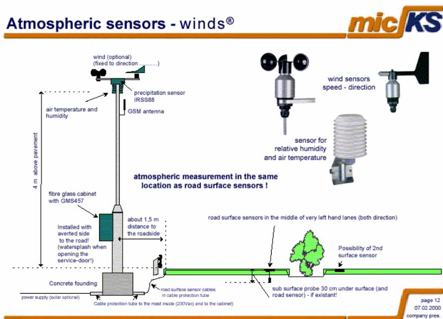
Figure 7. Road weather meteorological station scheme, taken from [5].
