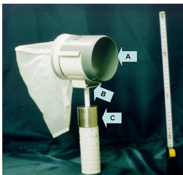
Fig. 2 Net-type snow trap (A), and mount (B). Part (C) contains the bearing. The trap mouth faces windward.
