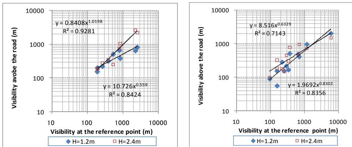
Fig. 6 Visibility at the reference point and on the roadway (left: flat, right: embankment)
