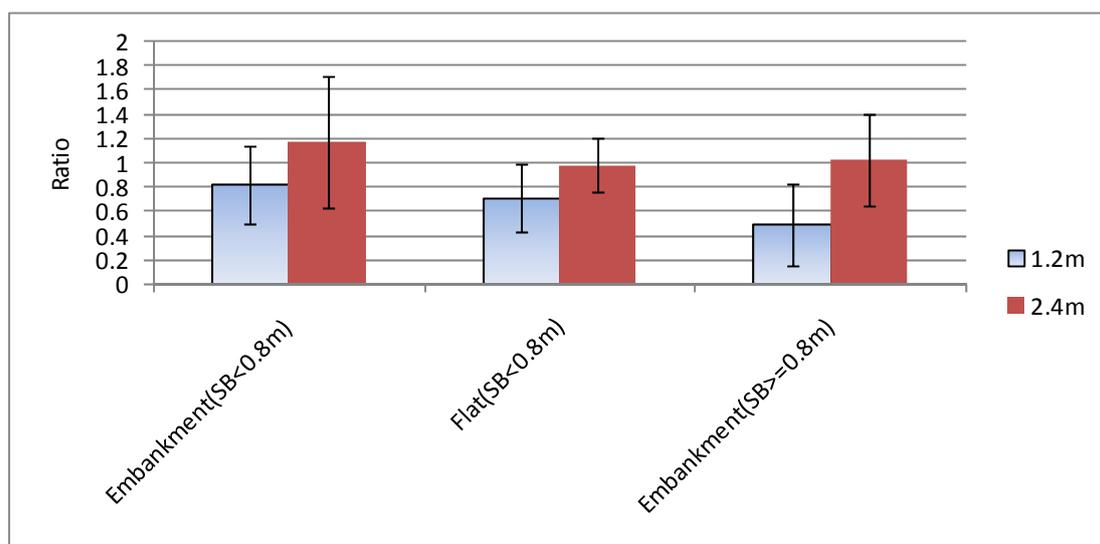
Fig. 5 Mean and standard deviation values of the ratio of visibility at the reference point to that above the roadway. SB means the height of snow bank.
