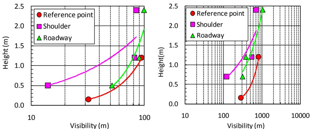
Fig. 3 Examples of measurement of visibility around the roads (Left: flat, Right: embankment). Height means the distance from the snow surface to the measuring height at reference point, and from the road surface at shoulder and roadway to the measuring height.
