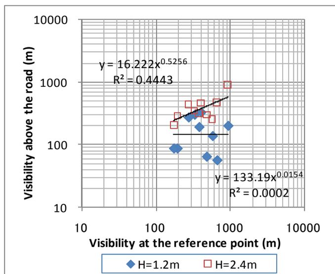
Fig. 7 Visibility at the reference point and on the roadway (embankment)
