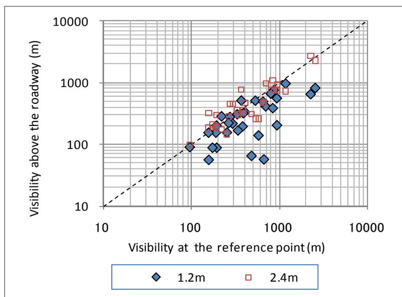
Fig. 4 Visibility at the reference point (1.2 m in height) and above the roadway (1.2 and 2.4 m in height)
