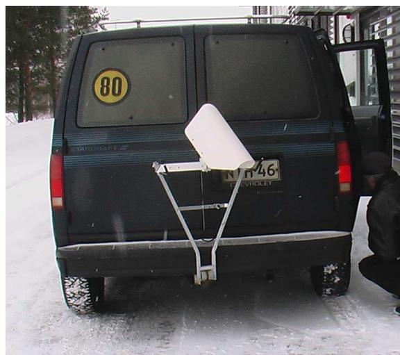
Fig. 3. Vaisala Remote Road Surface State Sensor DSC111 installed on a vehicle to measure mobile friction.
