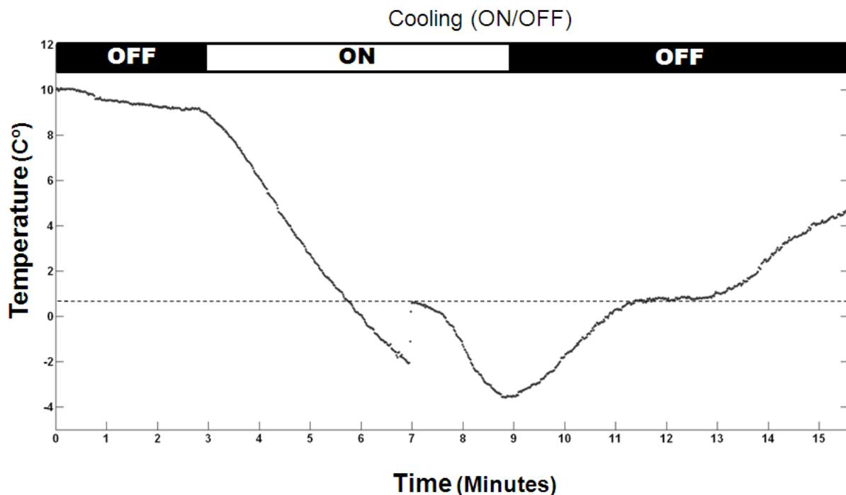
Figure 4. The temperature development during one cooling cycle with Active-BIRDS.
