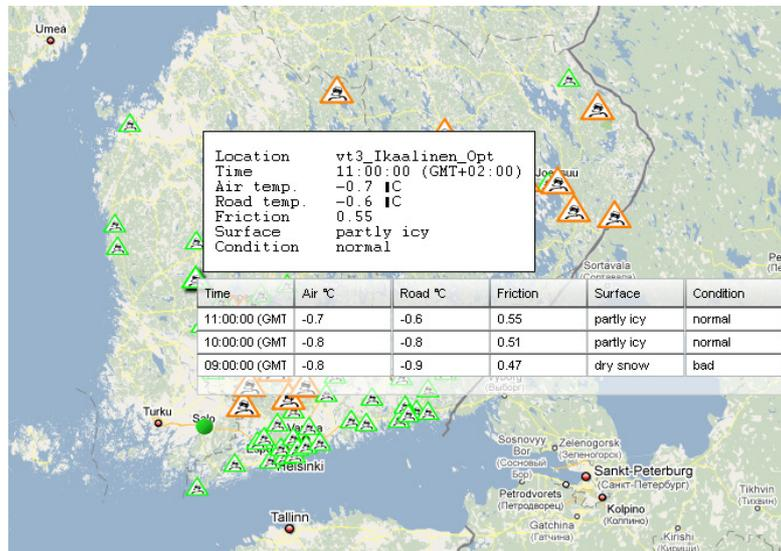
Figure 5: Forecasted friction and other road weather parameters presented in the Google maps ROADIDEA application. It based on close collaboration between ROADIDEA partners FMI, Destia and Demis.
