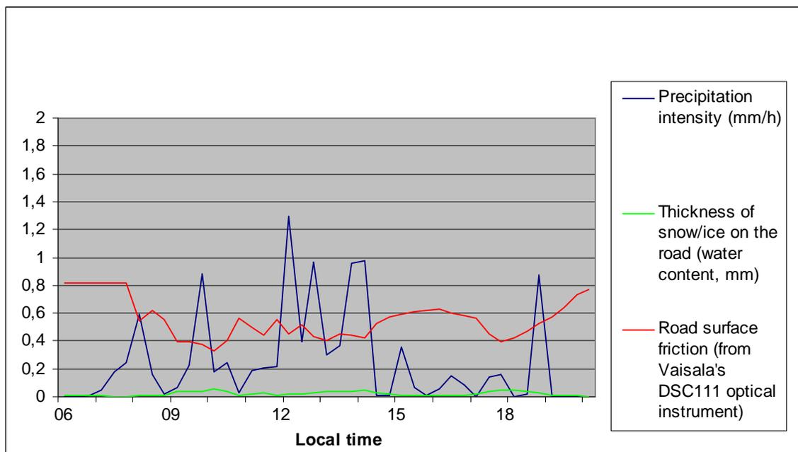
Figure 6. Road weather observations at Vaskisalmi station (about 4 km west of Helsinki city center) on 8 February 2007 06-20 local time: (a) air, road surface and dew point temperatures, (b) precipitation intensity, thickness of snow/ice on the road as well as road surface friction measured by Vaisala's DSC111 optical instrument (data source: the Finnish Road Administration).
