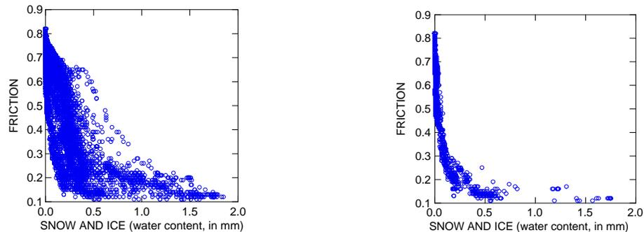
Figure 7. Scatter plot of friction vs. the sum of snow and ice (water content in mm) on the road. Based on DSC111 observations in Utti (in southeastern Finland) during winter 2007/08. The left figure includes all observations, the right figure covers those cases when road surface temperature was below  $-5^{\circ}\text{C}$  (data source: the Finnish Road Administration).
