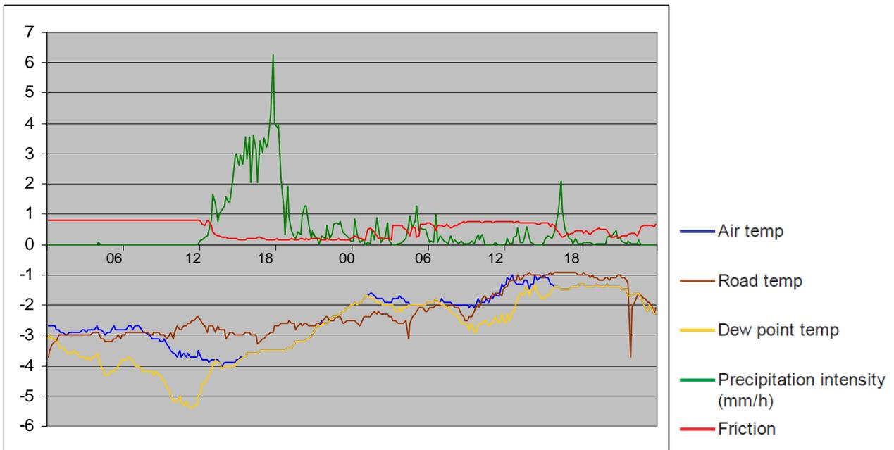
FIG. 3: Road weather observations at Palojärvi on a) 10-11 November and b) 23-24 November 2008. The measurements include road surface friction measurements by Vaisala's DSC111 optical instrument (Finnish Road Administration).
