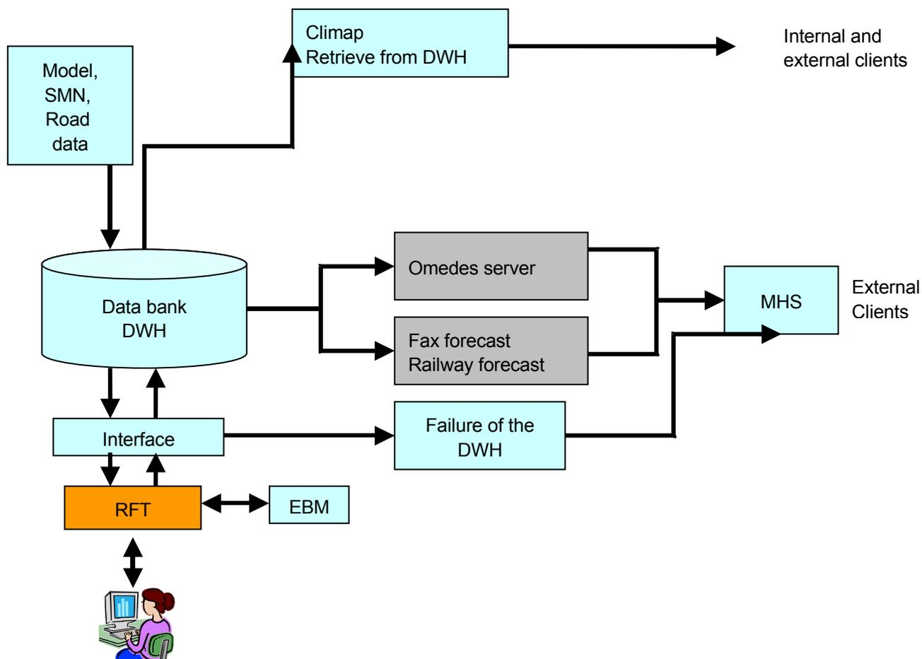
Fig 2: Flux of data associated with the RFT.
