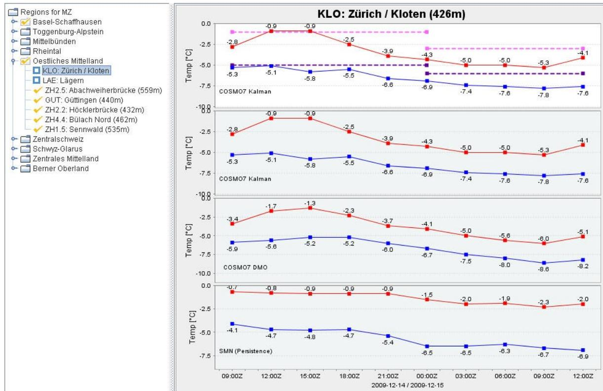
Fig 3a: The most appropriate 2 m temperature and 2m dew point curve is chosen between persistence, direct model output or filtered data.
