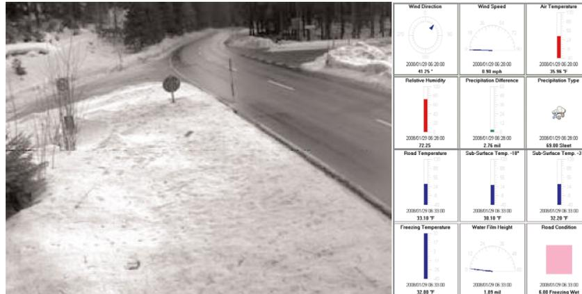
**Figure 6 Example picture and indicator display of data from a road site in Bavaria**
