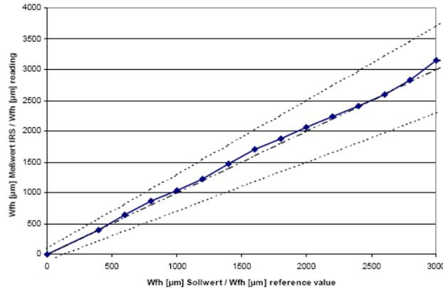
**figure 3 – Measurement characteristic of the microwave radar transducer in the passive road sensor**
