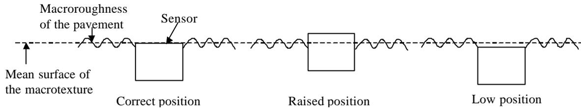
**Figure 4 : Positioning of a sensor in the pavement**
