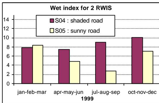
Figure 3 : Seasonal calculation of the wet index for two RWIS placed in very thin asphalt surfacing concrete
