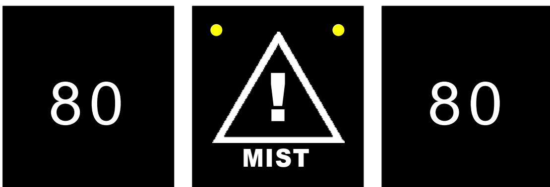
Figure 2. Representation of Matrix Signs of a Fog Warning System in the Netherlands.
