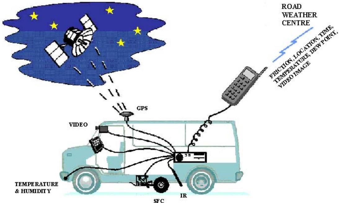
Figure 1. Basic drawing of the road weather meter.
